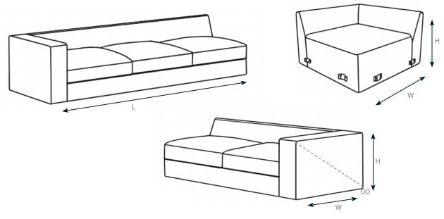
Length L must be less than entryway dimension 1, stairway dimensions 5, 4, & 3 and all interior doorway 7 or 8.
