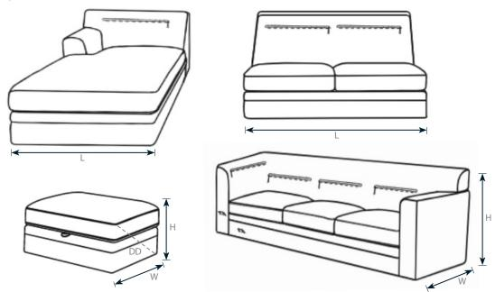
Length L must be less than entryway dimension 1, stairway dimensions 5, 4, & 3 and all interior doorway 7 or 8.
