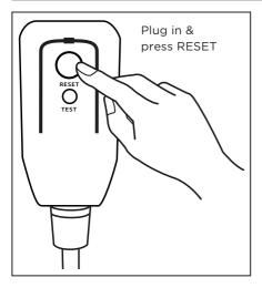
The power supply cord contains a current device that senses damage to the power cord. Test your power supply cord as follows:
