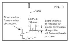
Add wood as shown in Fig. 11, or remove storm window before air conditioner is installed.
