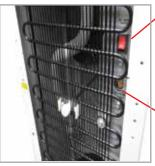
Adjustable cold water thermostat – factory set for maximum efficiency
