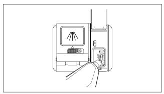
**NOTE:** Use the viewing port when filling the rinse aid reservoir.
