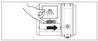
NOTE: The flap is always open at the end of a dishwashing cycle.
