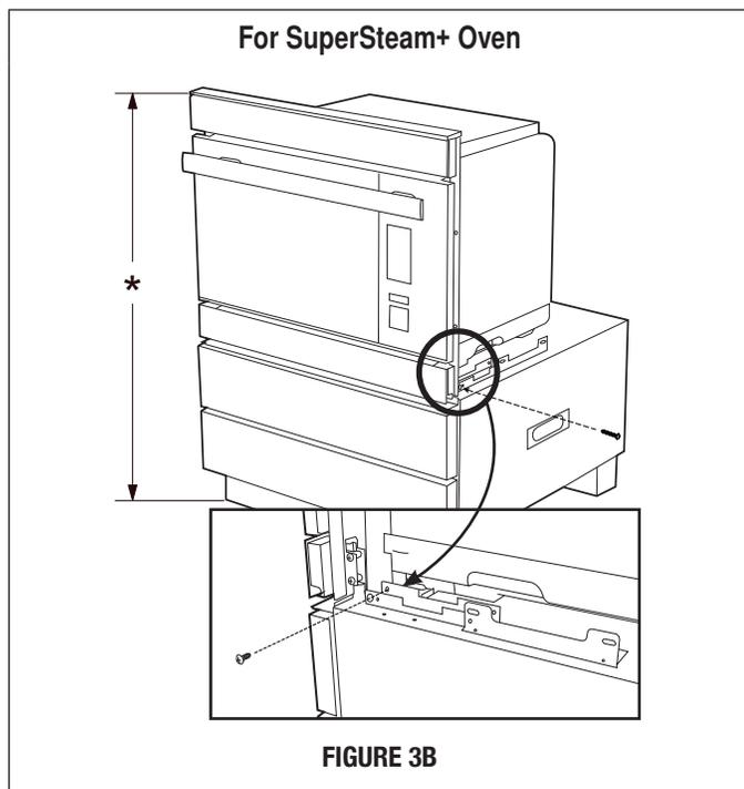
4. Adjust the height of the overall unit to fit your specific opening. The pedestal contains 4 adjustable feet. To adjust, have one person tilt the unit to one side while the other person adjusts the 2 feet on the raised side to the desired height. Repeat this step by tilting the unit to the other side and adjusting the other 2 feet. Ensure that all feet are adjusted equally to balance the unit. See Figure 4.
