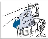
1. Press the Dirt Tank Release Button and pull away from vacuum.
