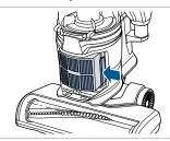
2. Press tab on right side of filter and pull out to remove from vacuum. Remove debris from filter by tapping on the side of a trash container. This pleated filter may NOT be washed.
