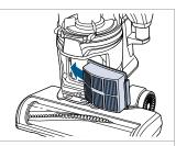
3. When reassembling, be sure to lock the filter back into place by aligning one side of the filter first, then clicking the other side into place.
