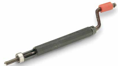
TYPE II Prewinder Prewinder reduces the diameter of the insert to that of the tapped hole allowing for easy installation.
