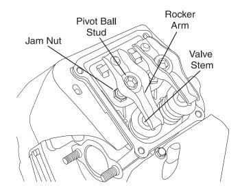
When valve clearance is correct, hold the pivot ball stud in place with the allen wrench and tighten the rocker arm jam nut. Tighten the jam nut to 174 in-lbs. torque. After tightening the jam nut, recheck valve clearance to make sure it did not change.
