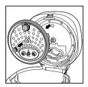
To assemble the detachable inner lid, fully attach it to the top lid, and then screw the nut around the temperature controller clockwise.
