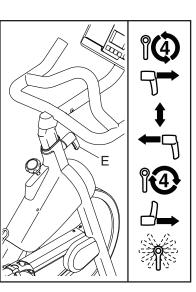
Make sure that the adjustment handle is engaged in an adjustment hole. Then, pull the adjustment handle outward, turn it so that it points downward as shown, and then release it.
