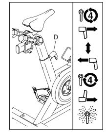
Make sure that the adjustment handle is engaged in an adjustment hole. Then, pull the adjustment handle outward, turn it so that it points downward as shown, and then release it.
