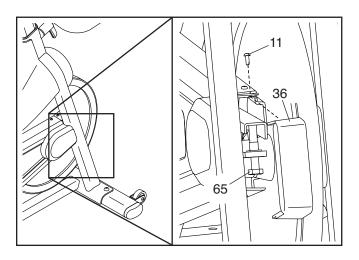
Then, tighten the M10 x 50mm Screw (65) until the Drive Belt (not shown) is tight.
