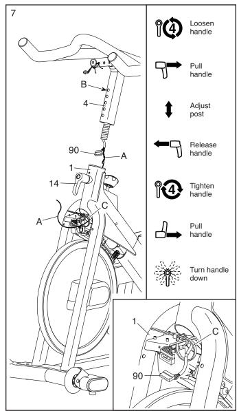
8. See the inset drawing. Connect the connector on the Upper Wire (90) to the connector on the Lower Wire (82). Tip: The wire connectors should slide together easily and snap into place with an audible click. If they do not, turn one connector and try again.
