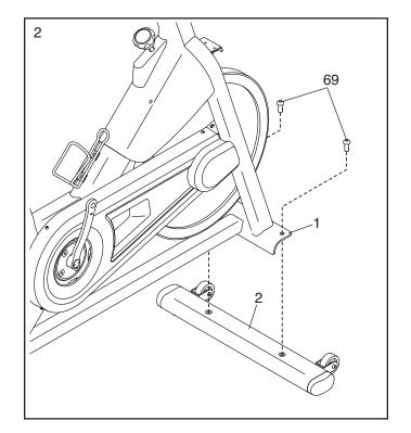
Attach the Rear Stabilizer (3) to the Frame (1) with two M10 x 25mm Screws (69).
