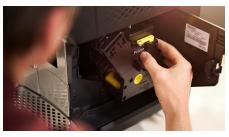
The brew group is the heart of every fully automatic coffee machine, and should be cleaned regularly. The removable brew group allows you to clean it thoroughly just by rinsing it under the tap.
