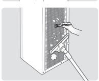
Remove the dust from the back of the appliance using a vacuum cleaner and soft brush.
