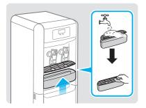
Remove the drip tray and grill from the appliance, wash it using neutral detergent and dry it using a soft cloth.
