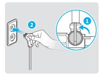
8 Drain water from the appliance completely via the cold and hot water faucets and drain cap. Repeat steps 7-1 and 8 more than three times to clean the inside of the appliance.
