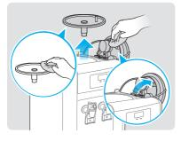
Close the angle stop valve and drain any remaining water via the cold and hot water faucets.
